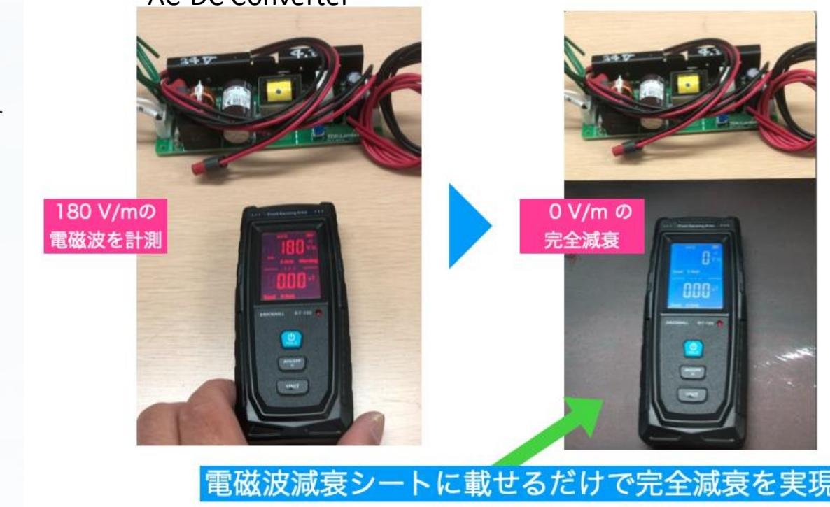
Achieves complete attenuation simply by placing it on the electromagnetic wave attenuation sheet
